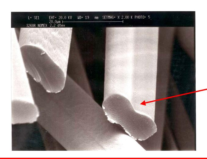
Capillary effect due to dog-bone shaped fibres
