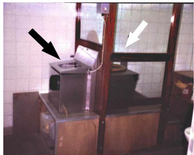
Fig. 3 Glass toilet, white arrow shows where the drug smuggler sits and black arrow indicates the part of the device where the containers are rinsed and cleaned (modified from Schaper et al. [17])
